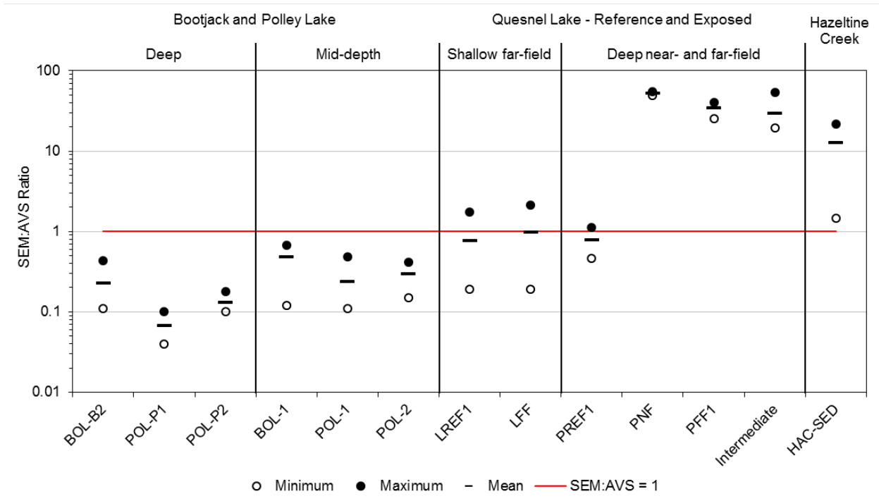
Figure 48: Summary of SEM:AVS Ratios for Sediments in Polley Lake, Quesnel Lake, and the Hazeltine Channel Sedimentation Pond
