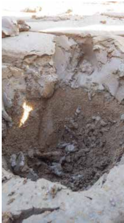
Photograph 11: View of ST15-04, showing two tailings types. Grey tailings are shown above magnetite sands tailings (September 13, 2014).
