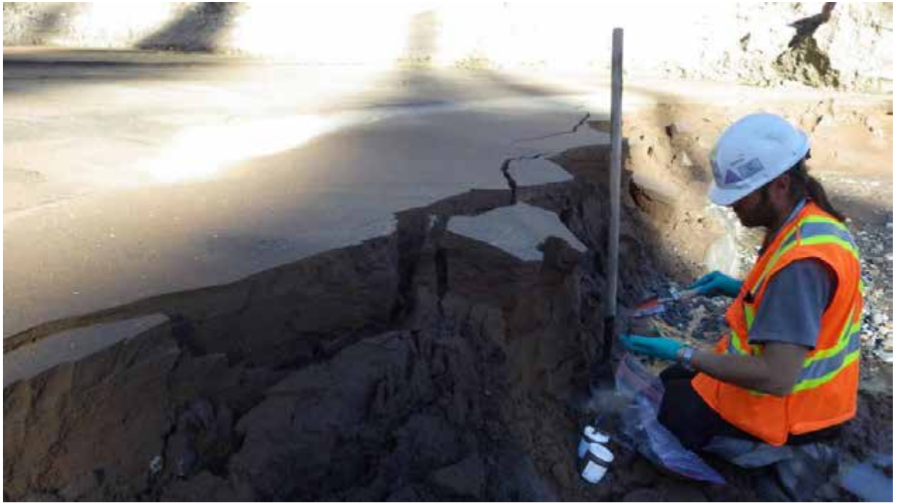
Photograph 17: View of ST11-02, showing a tailings sample being collected from a deeper deposit of tailings found in Upper Hazeltine Creek (September 14, 2014).
