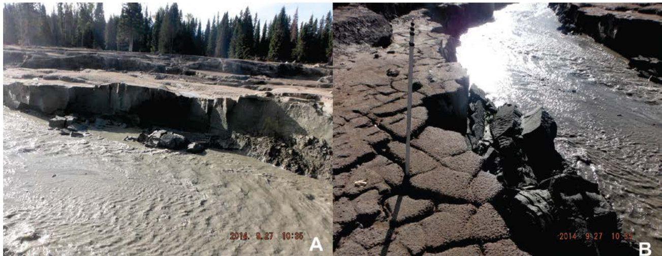
Figure 5-28: A&B – Hazeltine Creek right bank erosion of native glacial lacustrine material (HC-R9)
