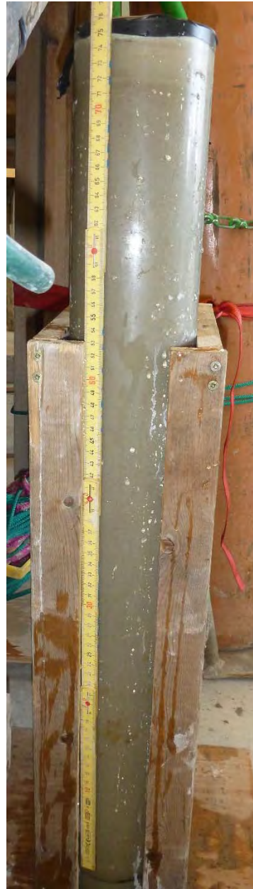
Figure E.33: Sediment cores collected from Quesnel Lake near field (QUL-PW-1) for profiles of pore-water (left core) and sediment chemistry (right core).
