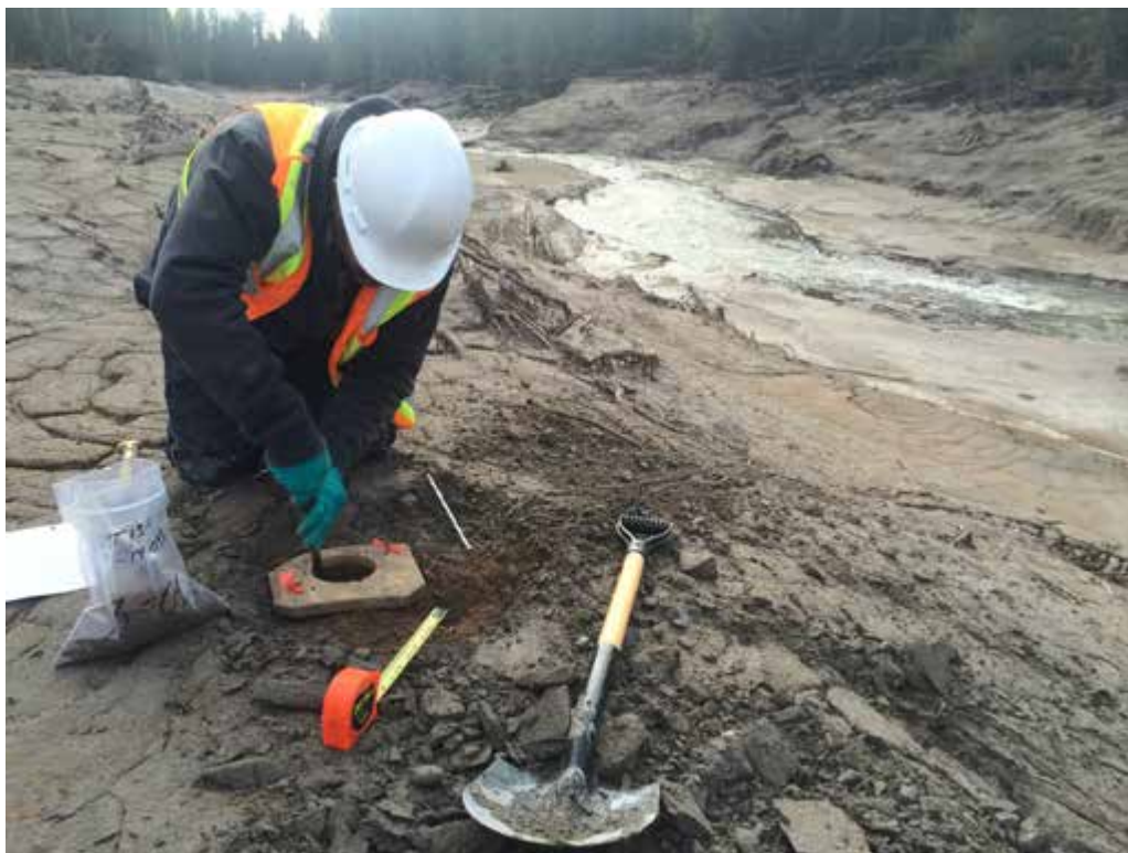
Photograph 18: View of ST13, showing a bulk density sample being collected (September 30, 2014).
