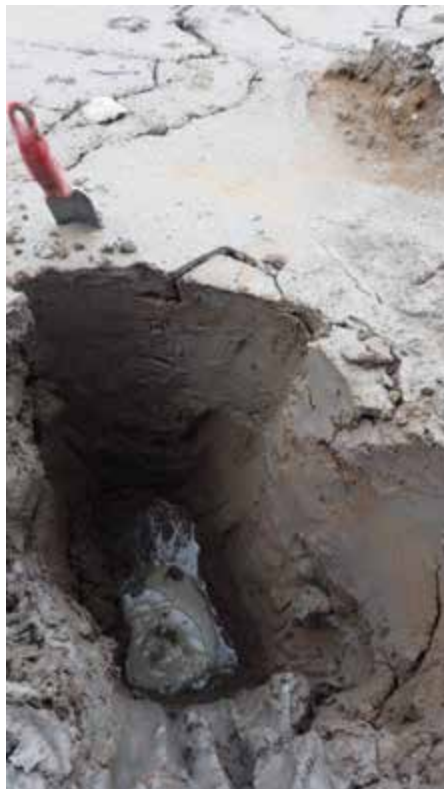
Photograph 10: View of ST18-02, showing tailings vertical variability near Polley Plug in Upper Hazeltine Creek (September 17, 2014).
