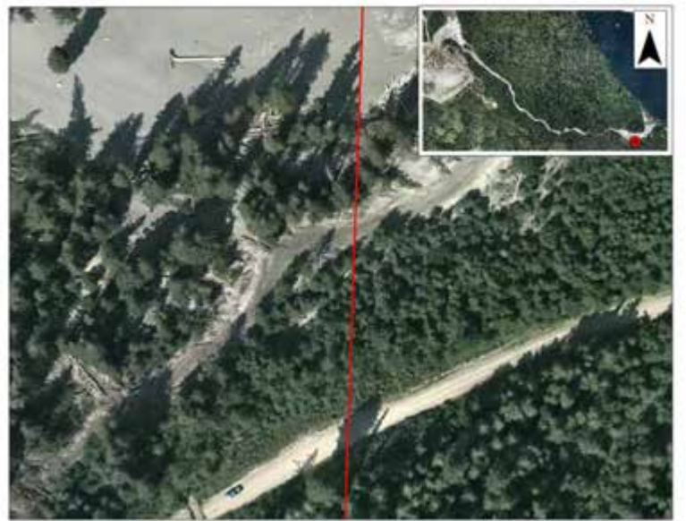
The affected area of Edney Creek extends 420 m upstream from the confluence with Hazeltine Creek. Near the confluence with Hazeltine Creek, Edney Creek is incised. Tailings are deposited within the channel above the incision.
