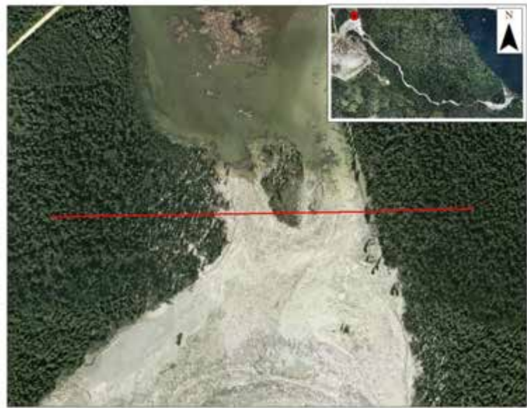
The Plug extends 1,750 m from the south end of Polley Lake. The area is dominated by debris flow deposits composed of tailings, native material and embankment material that span up to 350 m laterally.
