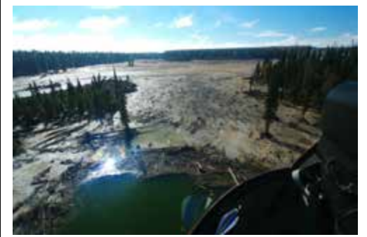
View looking downstream from Polley Lake. Fine grained tailings have been deposited across the wide floodplain to form the Plug.
