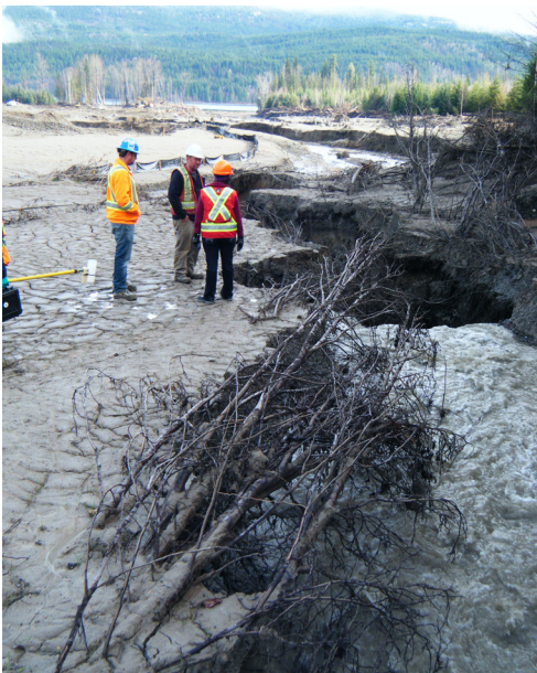
Slope instability and red tailings deposited within the Hazeltine Creek channel (September 22, 2014).
