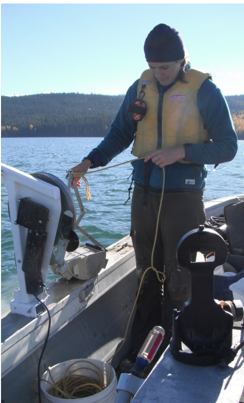
A scientist retrieves a sediment sample from the bottom of Quesnel Lake using a Petite Ponar device
