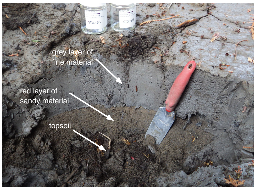
In some areas along Hazeltine Creek, the tailings settled in two layers over the native organic layer. The grey fine tailings settled out over the red-black sand. The concentrations of metals in the two layers were found to be similar.
