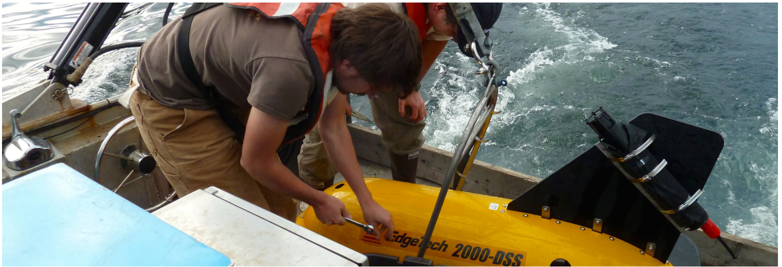
A sidescan sonar and sub-bottom profiler used to provide the acoustic “imagery” of the lake bottom and profiles of sediment layers beneath the lake.
