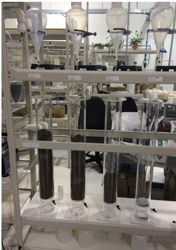
Figure 3-2: Column set-up at ALS Environmental. For scale, the diameter of the columns is 8 cm and the height of materials in column 1 (far left) is 45 cm.
