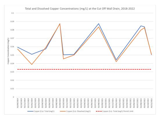
This graph shows the Cut-off Wall (COW) drain. Water trickles out, there is no substantial volume, but is above the permit limit. It drains into the breach sump which is 100 m upstream of the Perimeter Embankment Till Borrow Pond.
