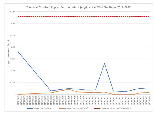
• This is the West Main Toe Drain: There are low concentrations of copper. We have the opportunity to send this water to the Water Treatment Plant, as it is amenable to discharge.
