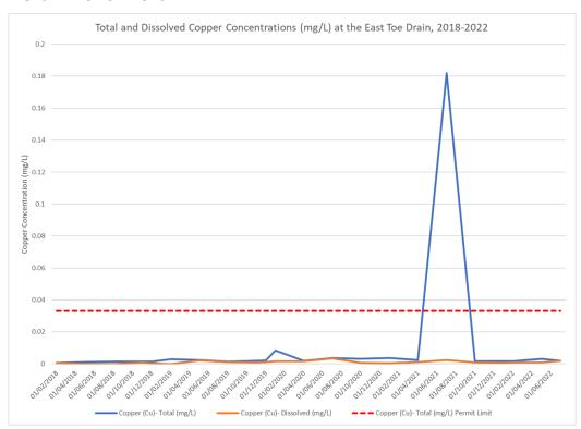
This is the East Main Toe Drain. It drains passively into main embankment seepage pond and the Tailings Storage Facility, where it is used for the sprinkler system. There is one outlier shown on this graph which is likely due to contamination or sampling error. We'll have to look at the filed data and the conditions at the time of sampling.
